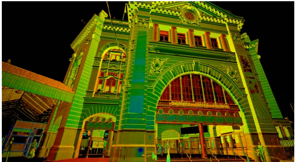
The custodians of Melbourne's Flinders Street Station use HDS technology to provide analysis on the buildings position, structural integrity and developments over time.
